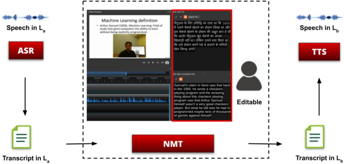
Figure 2.4 Block diagram of speech to speech translation. The transcript in language L_A is obtained from the speech using the ASR module, and then the text generated is translated into language L_B using the NMT module, which is editable by the user. The speech in language L_B is obtained from the translated transcript using the TTS module.
