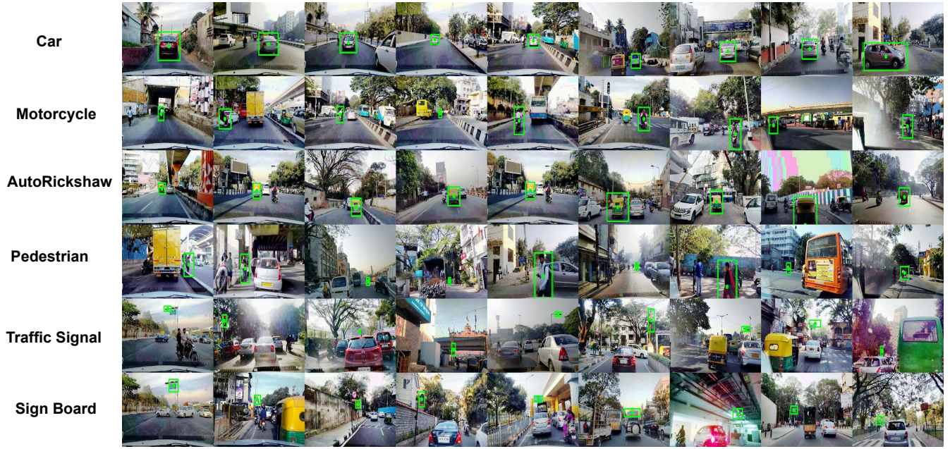
Fig. 3: Samples from DGAZE dataset corresponding to seven unique objects annotated on road. The samples are collected such that there is significant variation in the size of the object, distance of the object from the driver and illuminance variation on road.
