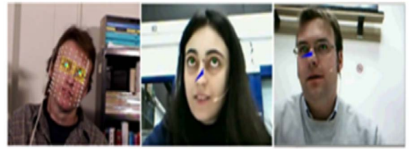
Fig. 2. (a) Combining cylindrical head model with eye-center locator. Yellow dots denote eye locations estimated by the view-normalized CHM, while green dots denote detected eye centers. (b), (c) Examples where gaze direction (green circle) differs from head pose (blue normal).
