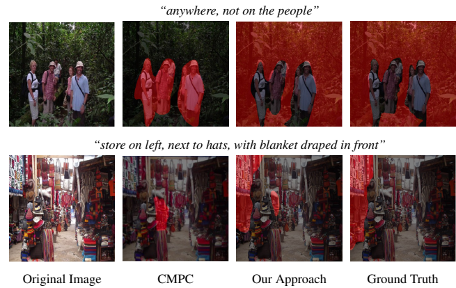
Figure 1. Comparison of the proposed approach with CMPC [8]. In both the examples CMPC fails at the first stage itself, where it completely misses the actual referred entity. Our approach performs the exhaustive forms of interactions in a single step and identifies the correct referred entity. Best viewed in color and under zoom.
