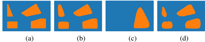
Figure 2. Decision boundaries of different networks trained for two class classification. (a) Original data: one class shown by blue and the other orange. (b) Decision boundary learnt using MLP. (c) Decision boundary learnt using IOC-MLP with single node in the output layer. (d) Decision boundary learnt using IOC-MLP with two nodes in the output layer (ground truth as one hot vectors)
