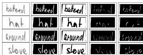
Fig. 5. Visualizations of the activations learnt by the 2nd convolutional layer of our network. The first column shows the pre-processed input image (taken from the IAM dataset). The second column shows the corresponding activations of a channel which acts as a textual edge detector. The third column shows a channel which activates on the image background. The fourth column shows a channel which acts like a vertical line detector, while the last column shows a channel which acts like a horizontal line detector.
