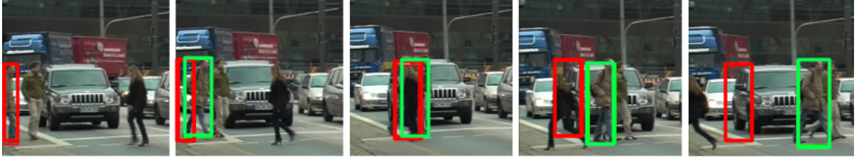
Figure 2: The behavior of proposed method ‘Collaborative Neighborhood Tracker’ in case of occlusion. First frame is the initialization frame and red bounding boxes are the initial tracking output. The algorithm selects middle frame as the key frame. After user annotation, the track updates (shown in green). Clearly, the tracking algorithm is handling occlusion well and the key frame selection is improving the overall track.
