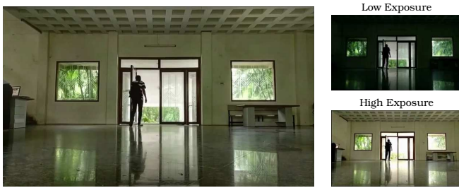
Fig. 7. HDR composition of a frame using two synchronous cameras with different exposure times.
