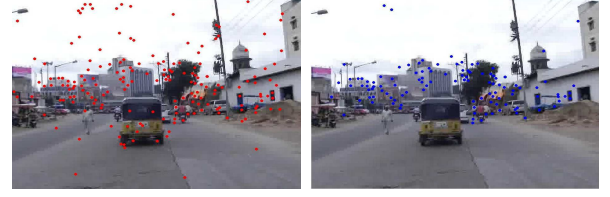
Fig. 4. The left image shows the visually stable features (matching static and dynamic elements) while the right image shows the spatially consistent features (static elements of environment).
