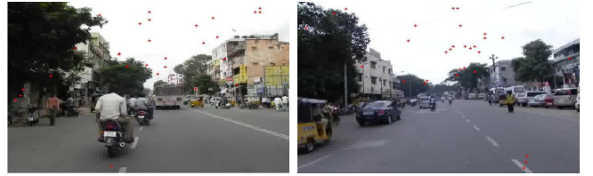
Fig. 9. Shown are the matching features from two sample frames returning large errors. The matching features correspond to non-distinctive elements like trees, sky and lane markings.
