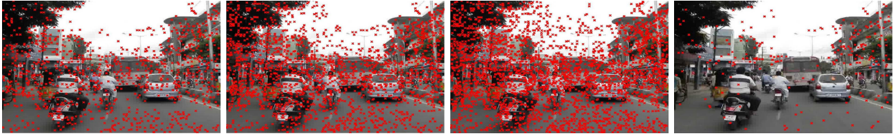
Fig. 5. Gradual learning of the useful features through base, augmentation and elimination run. Observe the growth in the number of features at a particular pose (from left to right) over run 1, 2, 3 and finally retention of only useful features in the last frame. Note that a small number of features in the last frame correspond to non-distinctive elements like sky. The effect of these features is negated using distinctive weights.
