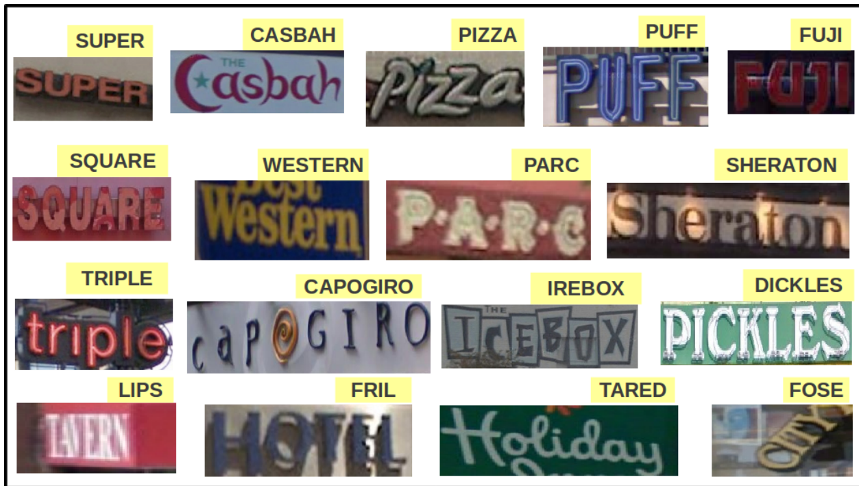
Figure 7: Example word recognition results on challenging images from the SVT dataset [29] using the node-specific lexicon prior. Our method handles many different fonts, distortions (e.g. CAPOGIRO in row 3). There are few failure cases however, as shown in the bottom row. We found the main causes of such failures to be: (i) weak unary term; and (ii) missing characters in the detection stage itself (see Figure 5). Some of these issues (e.g. CITY image in the bottom row) can be addressed by modifying the sliding window procedure.
