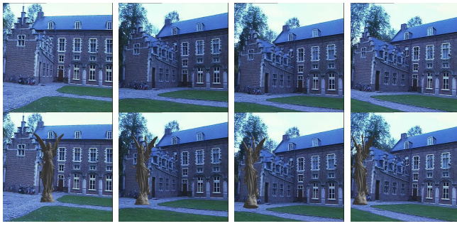
Fig. 4: Top Row: It shows the Leueven Castle sequence without the virtual object. Bottom Row: It shows the scene with the virtual object placed in the scene in front of the castle and moves accurately with the camera
