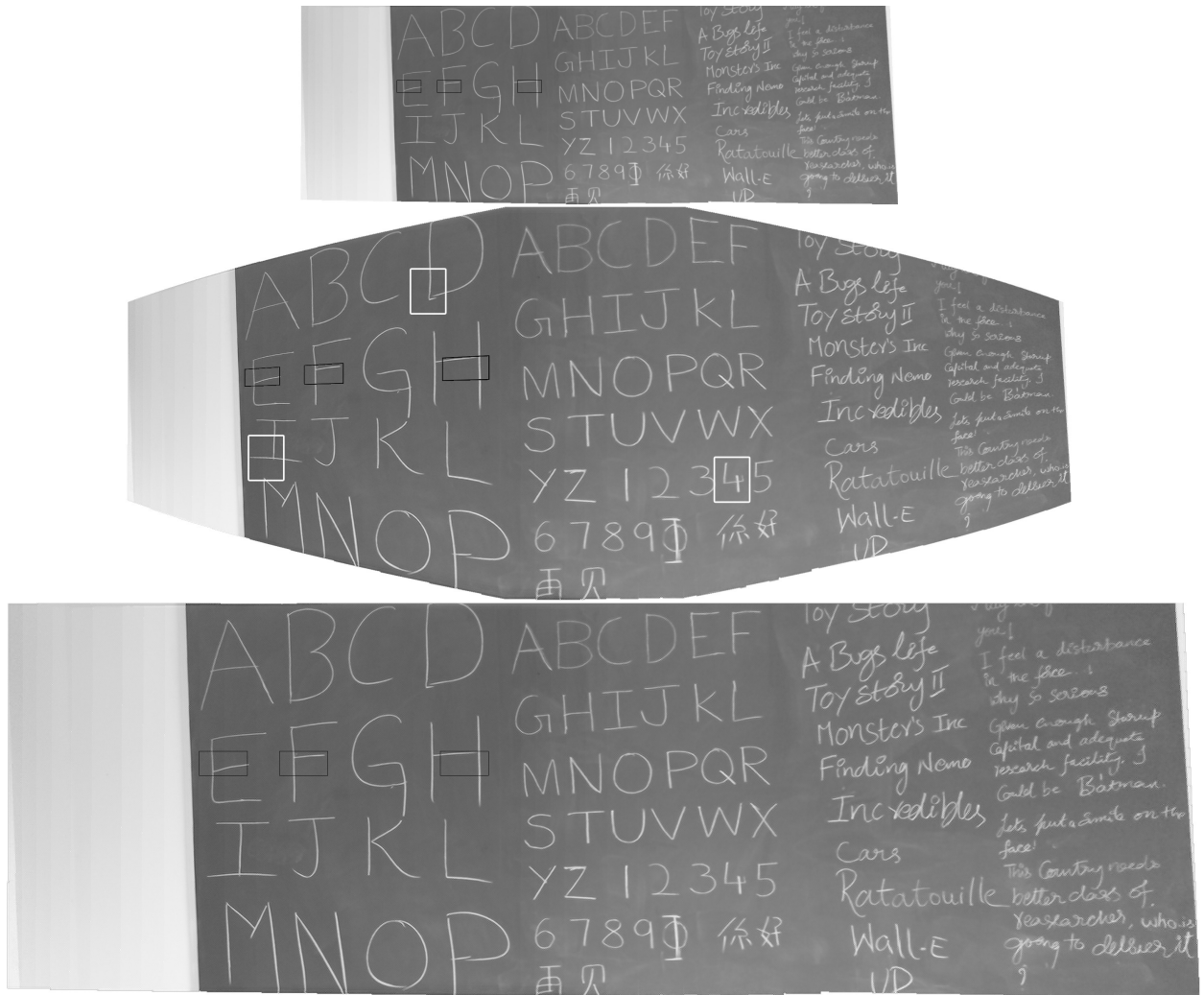
Figure 5. (top) Mosaic of the video sequence (1505 × 491). (middle) Attention based super resolved image output with a highest magnification factor of 2 (2370 × 982). (bottom) Mosaic super resolved by a constant factor (3010 × 982).
