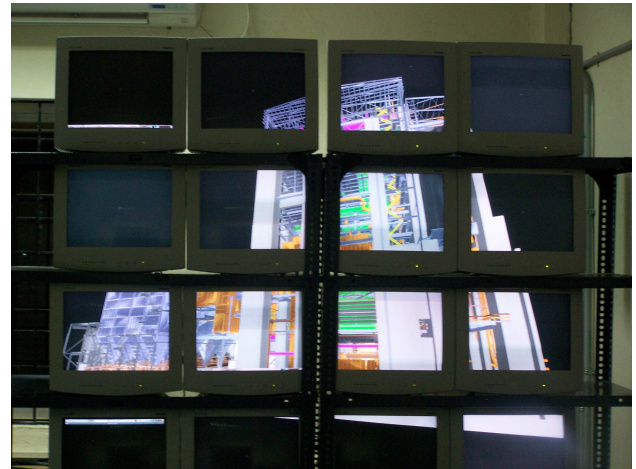
Figure 16: A 4 \times 4 display wall showing the Powerplant model. The combined resolution is 12 mega pixels.
