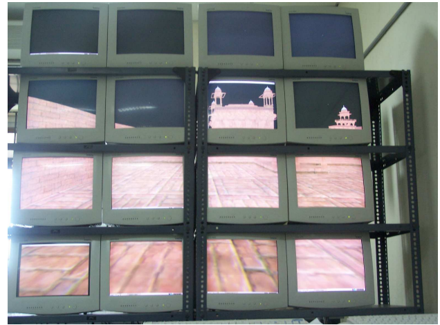
Figure 15: A 4 \times 4 display wall showing the Fatehpur Sikri model. The combined resolution is 12 mega pixels.
