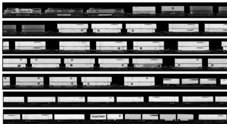
Fig. 6 (a) Velocity estimation; (b) assembling the centre sections of consecutive frame to form the panoramic image; and (c) example panoramic image of part of a train cut into multiple pieces for image display purposes
