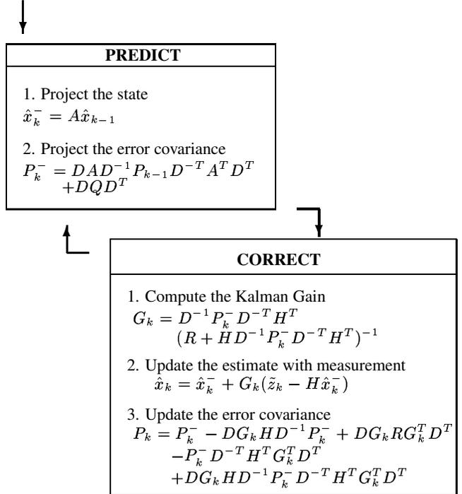
**Fig. 2.** Time update and measurement update equations for Two View Kalman Filter.
