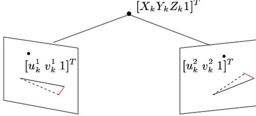
**Fig. 1.** The dark lines in black indicate the *actual* epipolar line, the dashed lines indicate the predicted epipolar line. The difference between these lines is denoted as the geometric error for that view.
