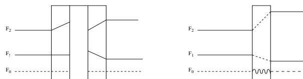
Figure 2: Illustration of formant transitions and pitch contours when the preceding vowel is different from the succeeding vowel. (a) V_1CV_2 for oral stop, and (b) V_1?V_2 for glottal stop
