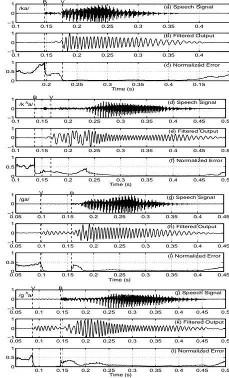
Figure 2: The speech signal, filtered output, and the normalized error for four different velar stop sound units
