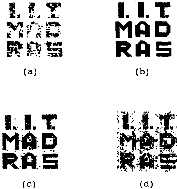
Fig. 4. Images reconstructed for different cases after 25 iterations. Original object: 128 \times 128 points; number of receiver elements: 128 \times 128 . (a) Only magnitude. (b) Only phase. (c) 2-bit phase with constant magnitude. (d) 1-bit phase with constant magnitude.
