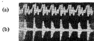
Fig. 11. (a) Voiced speech segment and (b) output of one-third octave bandpass filter centered at 10 kHz.
