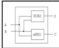
Figure 3. Design of the half adder
