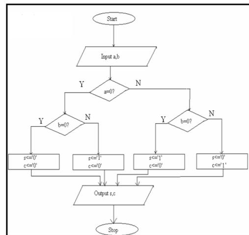
Figure 1. Flowchart depicting the behavior of half adder
