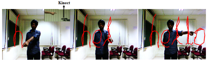
Fig. 1: User writes freely in front of a depth sensor (here Kinect). Our approach processes the trajectory and recognizes it in real time.
