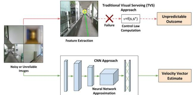
**Fig. 1:** Overview of the proposed *CNN Approach* compared to the *Traditional Visual Servoing (TVS)* used for autonomous corridor following. While the TVS approach performs well on clean images, it often fails to give a reliable output on noisy or occluded images taken from dynamically changing environments. The dotted line represents an unreliable step in the process. In such cases, a neural network can be used to estimate a desirable output.
