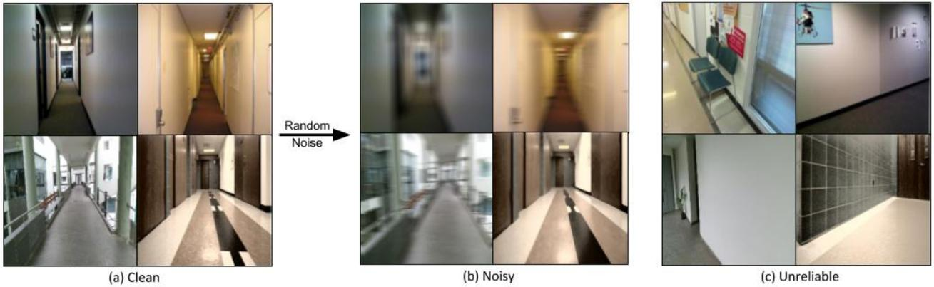
**Fig. 3:** Samples of images present in the dataset. The diversity in corridor environments can be observed in (a). Four different types of noises are artificially mixed with these images to obtain the noisy images shown in (b). Images where the required vanishing point features for computing the ground truth  $\omega$  could not be extracted are shown in (c). These have been discarded from training.
