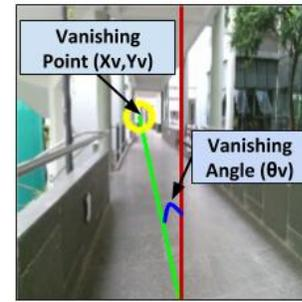
**Fig. 2:** Vanishing Point ( $x_v$ ) and Vanishing Angle ( $\theta_v$ ) features that are extracted by the TVS approach in [6]. These features are passed through a control law that computes a corrective velocity for autonomous corridor following. The red line is perpendicular to the corridor plane.
