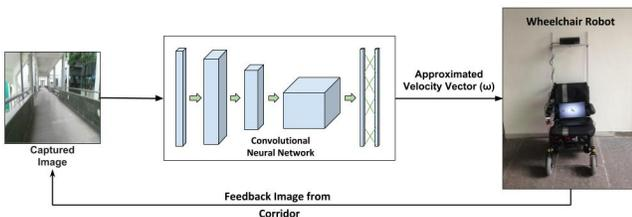
**Fig. 4:** Overview of our CNN Approach. An image captured from the corridor environment and passed through the CNN. The approximated velocity vector  $\omega$  is then used to perform servoing on the wheelchair.
