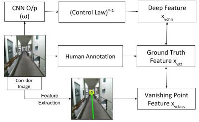
**Fig. 5:** Flowchart comparing Deep Features with TVS-based Vanishing Features. We perform a comparative analysis to understand why our CNN approach performs better in cases when feature extraction fails traditionally. This is achieved by extracting the  $x_v$  feature using both approaches and comparing them against a common human annotated ground truth.
