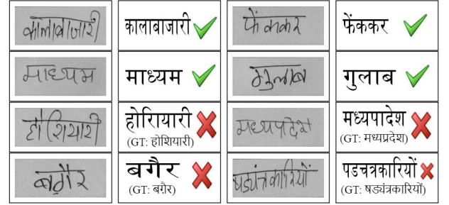
Figure 6. Qualitative results of the CNN-RNN Hybrid architecture on the IIIT-HW-Dev dataset. Here GT refers to ground truth.
