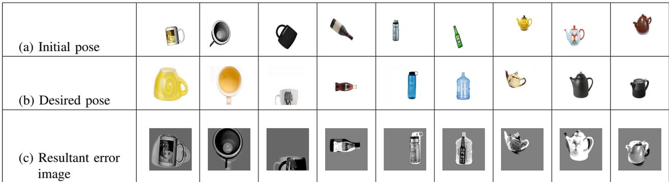
Fig. 5. **Qualitative results.** (a) Initial pose captured by the robot with a random camera pose for provided 3D object from the dataset. (b) Desired pose. (c) Resultant positioning compared to the desired pose by applying kernel SVM based visual servoing. Note the similarity in the resultant pose achieved by the proposed approach compared to the desired pose provided, over wide range of desired poses. Also note that, the selected 3D model in (a) acts as unseen target object.
