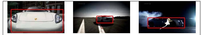
Fig. 1. Car detections from our approach in frames where [1] could not localize the same object with such accuracy. We use the localization in neighboring frames to interpret the location in any given frame, resulting in more accurate and faster detection.
