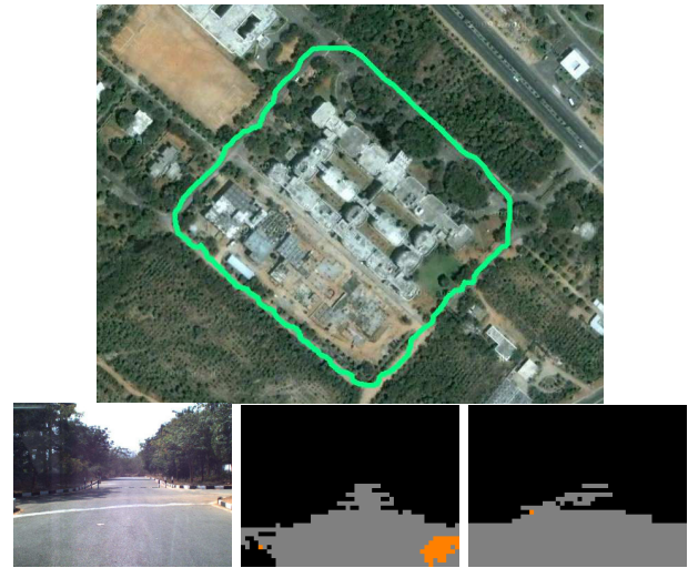
Fig. 7: 1 st row: Path navigated by robot in a closed loop, marked in green color. 2 nd row: Test image with predicted labelled images from the first and second loops.
