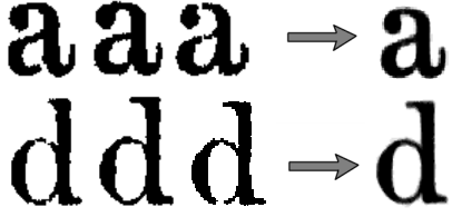
Figure 4. Collection of Characters and their Prototypes. A collection of 10 characters are used to generate the prototype.
