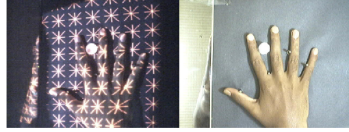
Figure 5. The hand under structured illumination as well as normal lighting. The mirror to the left enables us to compute height of palm at specific points.
