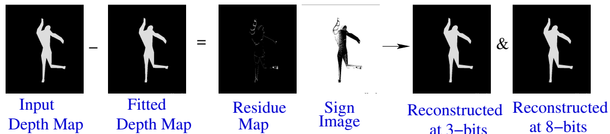
Figure 4: The input depth map, the fitted depth map, the generated residue and sign image, the reconstructed depth maps at 3-bits and 8-bits
