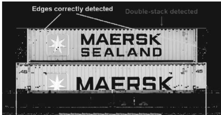
Fig. 7 Detection of gap boundaries (marked in blue) and identification of the object between the gap edges (marked with a red boundary to indicate a container)
