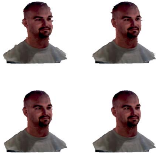
Fig. 3. [left – right, top – bottom] Novel views of the scene rendered with different quality factors [10, 20, 70, and 100] of JPEG compression. Edginess around the face due to JPEG compression decreases with increase in the quality factor
