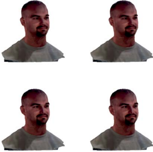
Fig. 4. [left – right, top – bottom] Novel views of the scene rendered when 0, 4, 7, and 12 bits from residues are added to the base depth map computed from polygonal proxy with 294 faces. Addition starts with the most significant bit. Rendering quality improves as the number of bits increases
